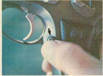
LEFT: Magazine release button is in exactly the right place for effective manipulation. trigger pull (in single-action mode) is smooth and polished.
